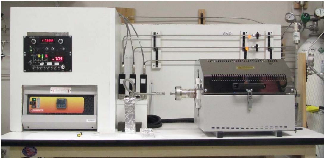
Figure 2.5 The home-built CVD graphene growth system
